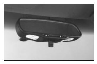
These lamps are located on the rearview mirror. Turn each one on and off by pressing its switch.
